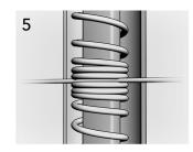
Push wire into the coils until they make contact with the Wire Centering Tool.
