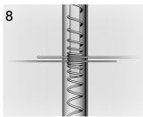
Add the next set of wires in the middle level coils and then the upper level coils. When installing a second wire into a set of coils, insert the second wire between different coils from the first wire.
