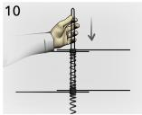
Squeeze clip and insert clip ends inside spring circumference and outside lateral wires to capture them. Slide all the way down.
