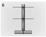
Repeat steps 4-5 to install the second wire in the upper level of spring coils.
