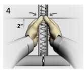
Place first wire between two coils at the middle level, leaving two inches of wire at the end of the spring. Keep thumbs close together on wire against coils and push the wire between two coils. Cut off the wire on the left at the 2" mark
