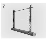
Install next spring at a maximum of 5' distance and repeat steps 3-6. Use the inserted wires from the first spring to complete the connection to the second spring.
