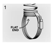
Locate the flat end of spring and insert clamp band between the 2nd and 3rd coils. Note: you can open the clamp first and then insert the band between coils.
