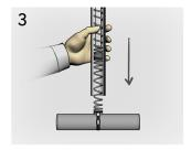
Place Wire Centering Tool over spring and slide down.
