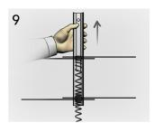
Once wires are installed in spring, remove the Wire Centering Tool. Adjust wires to center if necessary.
